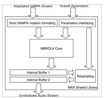
As shown in Figure 8, we can separate the possible requests in two main channels. On one side, there is parameter modification, which influences the internal state of the synthesizer. On the other side, there is the phonetic/prosodic stream, which generates speech instantaneously.
