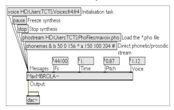
The MBROLA engine can also be stopped (*Messages* inlet). That function flushes the phonetic/prosodic content, stops the synthesis process and sets all the internal parameters to their default values. The diphone database remains loaded.
