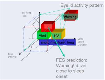
Fig. 14 A schematic of the FES premise space. Depending on which fuzzy rules are triggered by the eyelid activity pattern the output of the system is calculated in real time.
