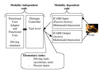
Fig. 5. Overall architecture of the multimodal driving simulator.
