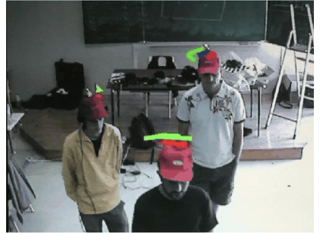
Fig. 9. IR tracking of the lights on top of the red hats (green), color tracking of the top of the red hats (red)
