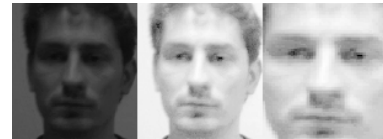
Fig. 14. a) The original captured frame, b) The illumination compensated image, c) The result of the adaptive cropping
