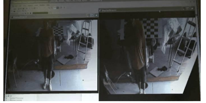
Fig. 8. Left: initial video frames, right: real-time projective warping using OpenCv-based EyesWeb block
