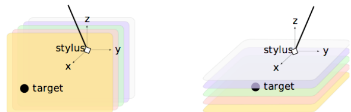
Figure 1: Virtual environment composed of a number of parallel planes positioned either horizontal or vertical to the phantom stylus.
