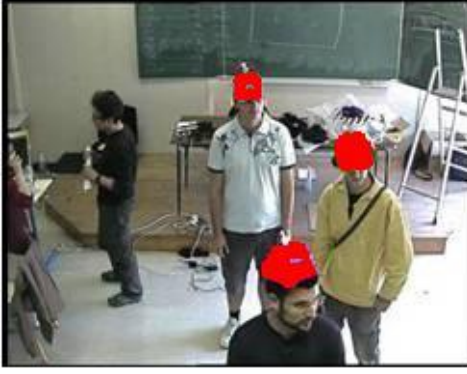
Fig. 3: Color-based red hat blob detection
