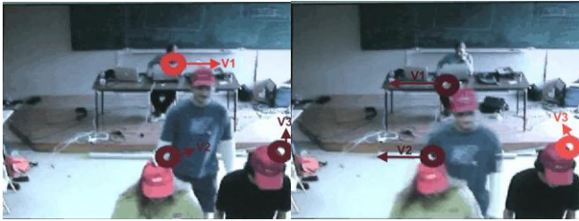
Fig. 11: Left: fastest moving object ( V_1 ) is the most important (hot red), Right: slower moving object ( V_3 ) is the most important.
